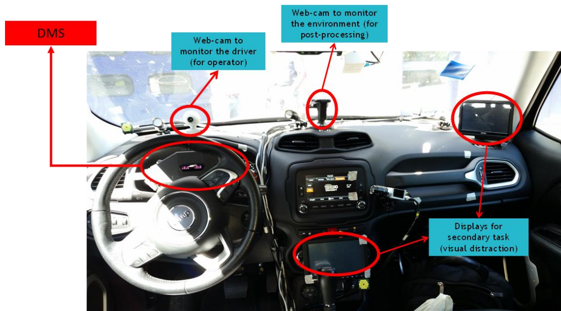
Figure 15: Cockpit Installation for the experimental set-up in test-vehicle.
