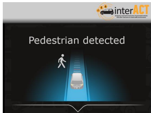
Figure 15: Example for the on-board HMI display.
