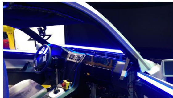
Figure 14: Integration of the 360° Light Band in driving simulator vehicle.
