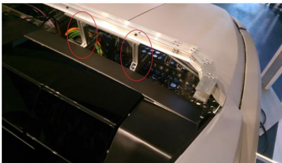
Figure 14: Integration of the 360° Light Band in driving simulator vehicle.
